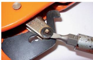
1. Remove the ratchet pin clip by levering up the edges with a small screwdriver (note: the clip is not to be used again)
