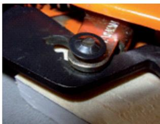
8. Place a thin support base under the head of the ratchet pin to stop it moving
