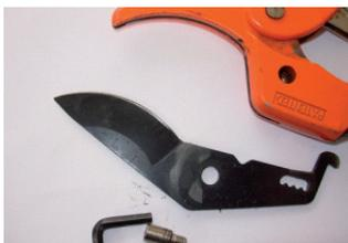
4. Hold the blunt edge of the blade and pull it forward to remove the blade
