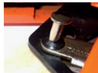
10. Use the supplied rivet and a hammer to tap down the clip
