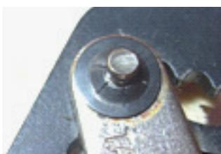
11. Ensure the clip is on the groove in the ratchet pin. Keep the allen key and all spare parts for future use
