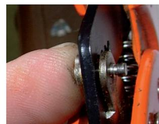
6. Insert the new blade and tighten the bolt with the allen key
