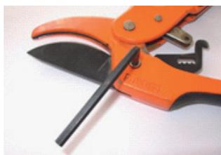
3. Undo the centre retainer bolt using the allen key supplied with blade kit, remove the bolt
